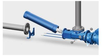
The reliable pump with cardan joint is excellent for conveying sludge in Wastewater treatment plants. Fast rotor/stator changes are possible thanks to the **patented** <u>WANGEN X-LIFT quick-change system</u> developed by the German company WANGEN PUMPEN. When removing or installing the rotor/stator, there is no need to remove the pump from the piping system thanks to its Service in Place design. The Xpress pump ensures easy maintenance and considerably shortens the servicing time.
